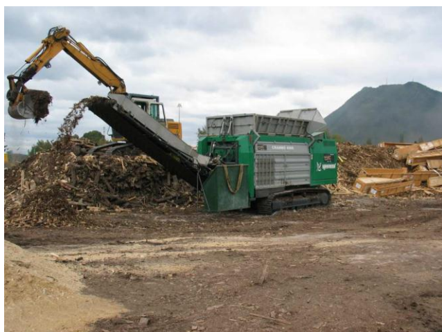
Figure 4: Crambo 6000 turning stem off-cuts, bark and packaging waste into boiler fuel.
