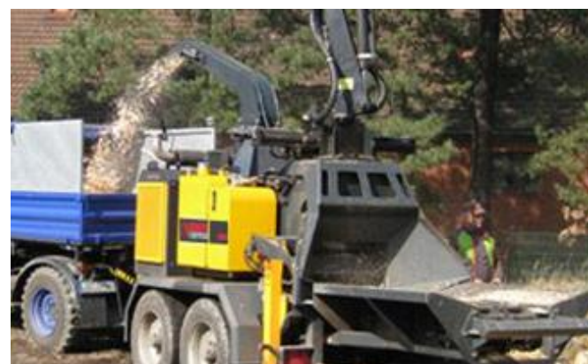
Figure 3: Small trailer-mounted drum chipper, limited to material less than 41 cm diameter.
