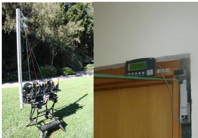
Figure 1: UC Model Yarder and load cell with custom built mounting bracket for measuring skyline tension.
