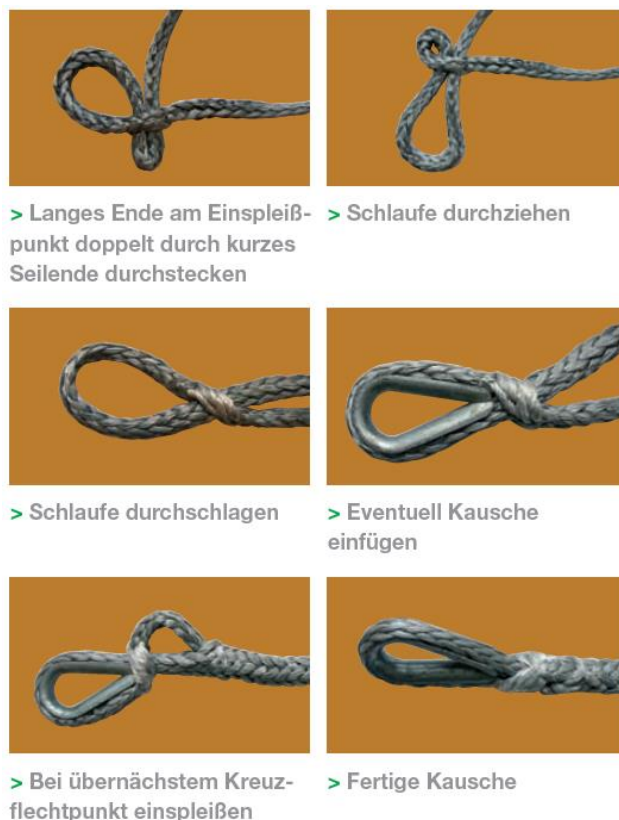
Figure 4: Example guidance on rope splicing (Ossiach Forest Training Centre resources).
