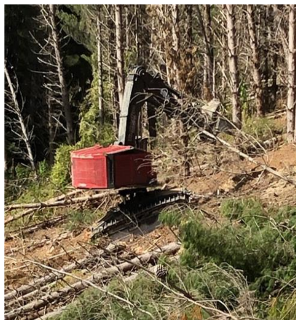
Figure 1: TimberPro 765 feller buncher with Komatsu KS800 fixed wrist felling head
