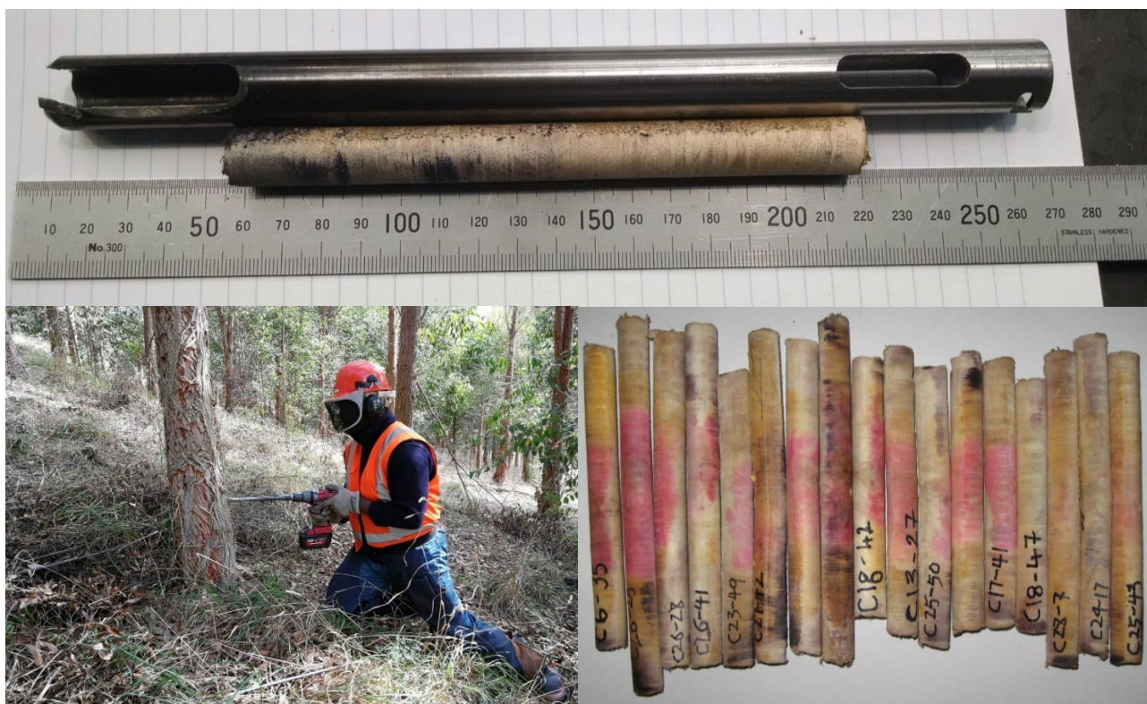
Figure 1: Top: corer developed by Callaghan Innovation to extract bark-to-bark stem cores with a diameter of ~14 mm from high density eucalypts. Bottom left: Coring an E. globoidea tree using a light-weight battery powered corer. Bottom right: labelled E. bosistoana cores with heartwood highlighted pink through staining with the methyl orange pH indicator.
