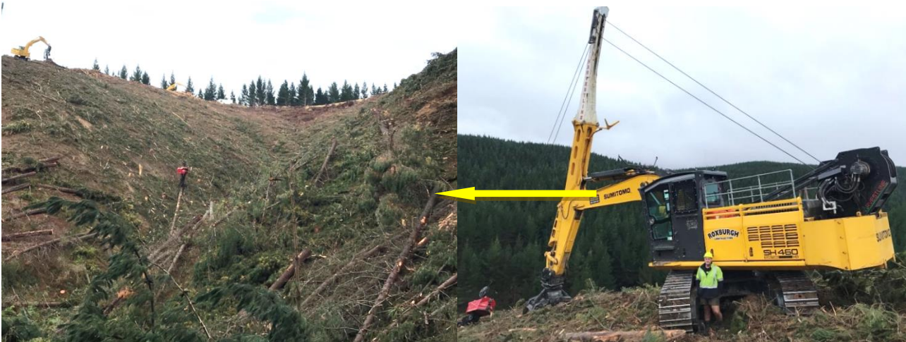
Figure 4: Left - Harvestline working across the gully with good deflection, and Right- Harvestline with operator Blair.
