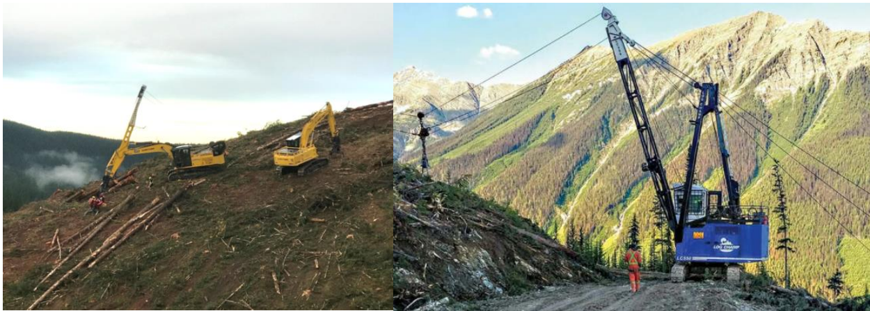
Figure 2: The excavator based HarvestLine (left) is able to operate, in comparison the much larger full size swing yarder (T-Mar 650 shown on the right) requires a good level landing location to operate.
