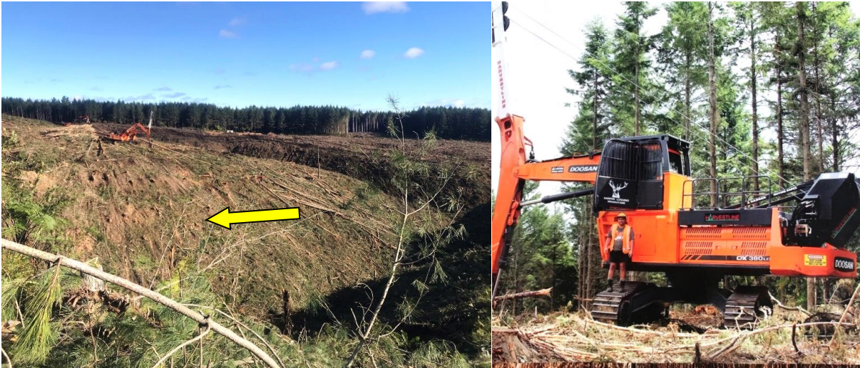
Figure 5: Left showing the direction of work across the slope and right the Harvestline with operator Hemi.
