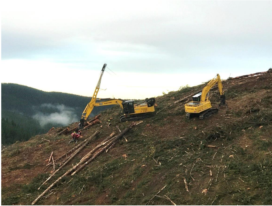
Figure 17: In Mosgiel, the Harvestline operator moved down off the main landing to improve deflection and cycle time. The excavator-grapple machine shovelled the extracted stems up to the landing.
