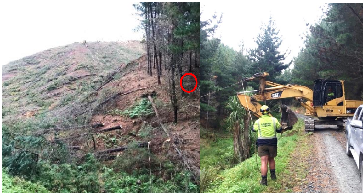
Figure 5: The extracting corridor as seen from the road (left, on which the tail hold was located (right). Another important aspect seen here is the broken terrain, through which logs were pulled over.
