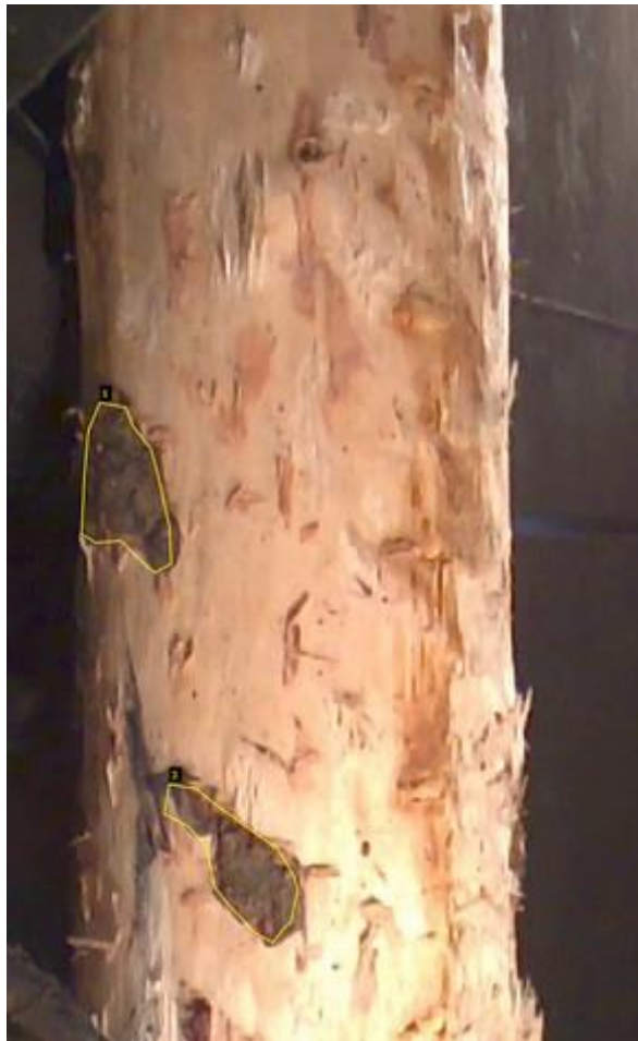
Figure 1: Example of a log image that has bark regions manually annotated for training.
