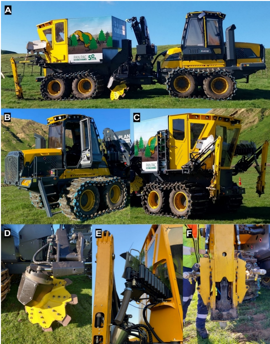
Figure 1. The Plantma Forestry PlantMax. A, an overview of the PlantMax. B, the Eco Log 574E forwarder. C, the planting module. D, one of two Midiflex scarifiers. E, seedlings loaded in a carousel prior to being released into the planting arm. F, a planting arm head with mounted spray nozzles.
