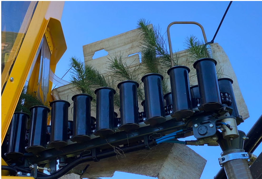
Figure 20. Forester ingenuity. To combat wind on the planting sites bending the seedlings and causing mechanism feeding issues, sections of planting box were cable tied against the seedling carousels to act as wind breaks.
